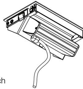
Attach 1 clips, at each end of unit base.
