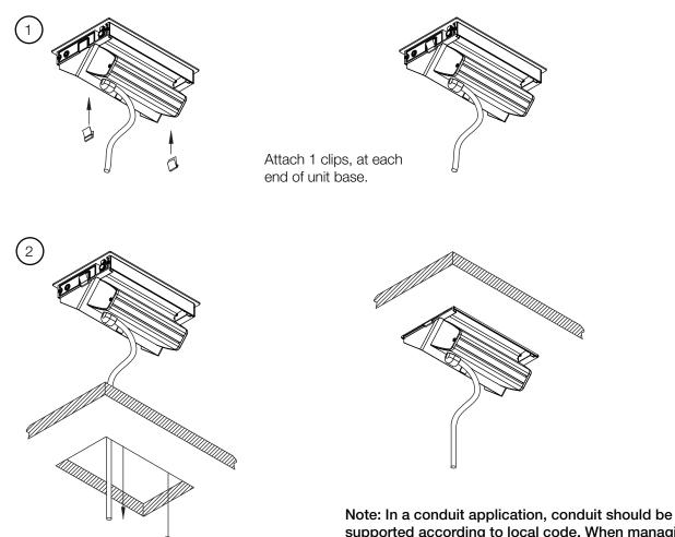
Note: In a conduit application, conduit should be supported according to local code. When managing conduit and cabling exiting the unit, ensure there is adequate slack to allow unit to open properly
