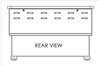
/1/2" BOARD IN BACK TO ATTACH CUSTOMERS OWN ELECTRONICS CAN BE REMOVED IF NOT NEEDED IN THE FIELD.
