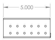
DIMENSIONS ARE IN INCHES TOLERANCES: FRACTIONAL±1/32 ANGULAR: BEND±1° ONE PLACE DECIMAL ±.02 TWO PLACE DECIMAL ±.01 THREE PLACE DECIMAL ±.005
